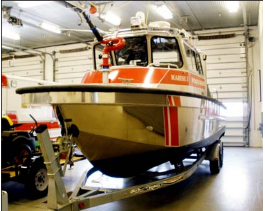
New 27-foot all-aluminum North Wind marine boat, manufactured in Seattle, Washington. Arrived in mid-January.
